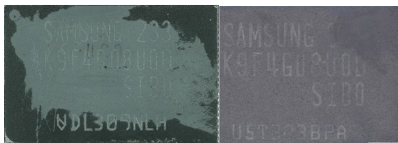
Figure 29 Resurfacing Comparison of Large vs. Small Processed Area
